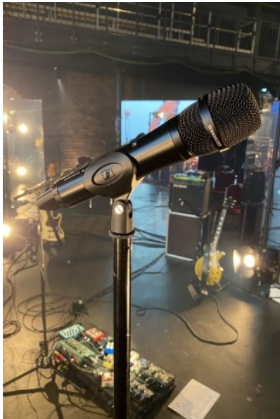
Milliarden’s Ben Hartmann used an evolution wireless 500 G4 handheld transmitter with the new high-rejection MM 445 microphone head
